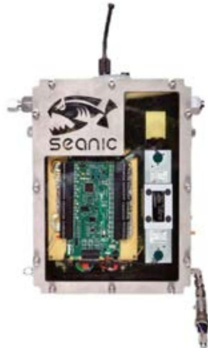
The 5 Station Intelligent Valve Pack can be configured to meet many requirements. The pack is designed and built to operate our smart torque tool, but can also be configured for other tooling requirements including flots and custom multi-functional tool.
