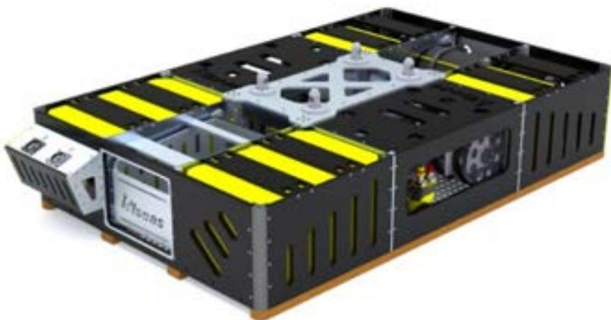
The ROV Tooling Skid is suitable for connection to most work class ROV's. The pin configuration is to fit the Forum XLX & UHD ROV systems as standard. The Skid is constructed from a lightweight aluminum frame and has been designed to maximize available space whilst still providing positive buoyancy. It is protected with removable HDPE panels for ease of access.
