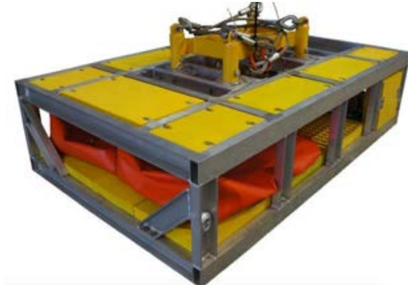
The standard ROV Tooling Skid is suitable for connection to most work class ROV's. The pin configuration is to fit the Triton XLX ROV as standard but can be adapted to any other work class ROV. The Fluid Injection Skid is designed for various pressure testing and fluid injection applications subsea. It comes with a proportional 0-10,000 PSI IHPU and is designed to be used with a client provided Hot Stab.
