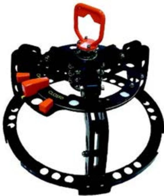
The Mechanical VX- Ring Tool is a mechanical tool without use of hydraulics or electric power. The tool is designed to land on top of the wellhead or XT. By operating the open/close handle the tool will release or grab the VX-Ring. The tool allows bore protector to be fitted on XT when installing or removing the VX-Ring.
