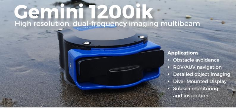
The Gemini 1200ik multibeam sonar operates at two acoustic frequencies, 720 kHz for long range target detection, and 1200 kHz for enhanced high-resolution imaging. The sonar maintains a wide 120° horizontal field of view when operating at both acoustic frequencies.
