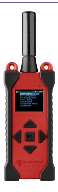
The iWand is a handheld acoustic transponder test and configuration device developed for use with Sonardyne's 6G® product range.
