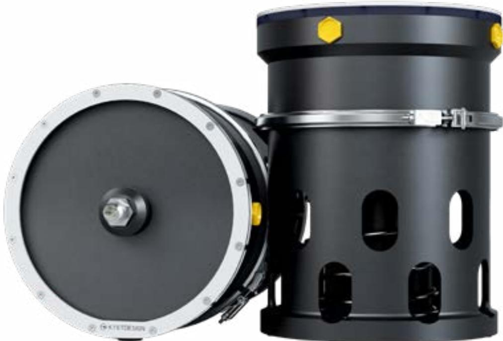
The function of the compensator is to maintain a raised pressure in a fluid circuit related to ambient at all water depths. This is achieved by a spring acting on a rolling diaphragm, i.e. the connected fluid circuit will always see a pressure equal to ambient sea water pressure plus the pressure generated by the spring.
