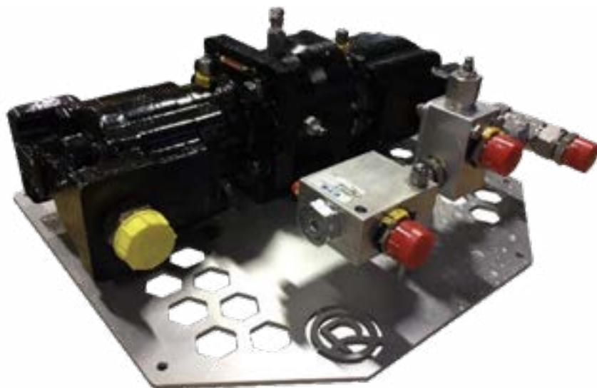
The 100 L/min Dirty Work Pack is designed to protect the hydraulic circuit of the ROV against external contamination during fluid transfer operations. It utilises a hydraulic motor powered by the ROV hydraulic circuit to drive a pump which supplies the delivery fluid from an external compensated reservoir.
