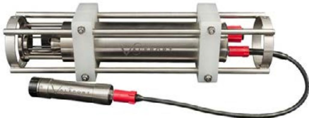
The MIDAS BathyPack is one of Valeport's premier MIDAS products, using state of the art sensors to generate precision Sound Velocity and Density profiles for highly accurate depth and height data. The simple top-end PC software, BathyLog, also allows all profile data to be used to monitor and correct multiple miniIPS pressure sensors, giving you the complete picture with one integrated sensor suite.
