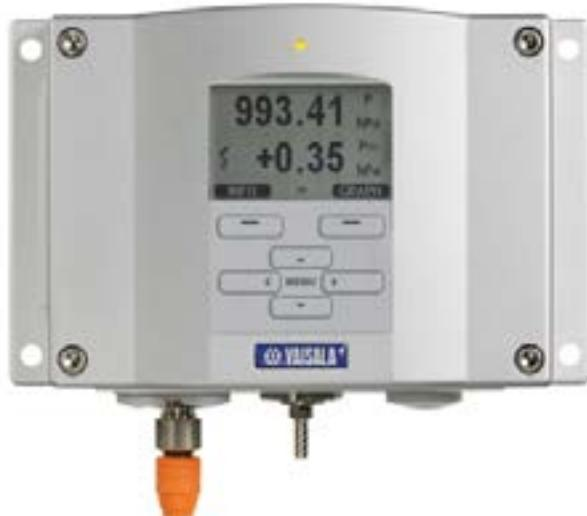
Vaisala BAROCAP® Digital Barometer PTB330 is a new generation barometer, designed for a wide range of high-end atmospheric pressure measurement. The pressure measurement of the PTB330 is based on the Vaisala in-house, silicon capacitive, absolute pressure sensor the Vaisala BAROCAP® Sensor. It provides high measurement accuracy and excellent long-term stability.
