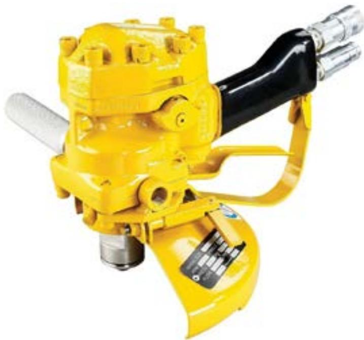
The GR29 is a widely used and industry recognised multi-purpose cutting, grinding and cleaning tool for underwater operations used by ROV's and Divers. It has a variety of attachments and is driven by a high torque gear motor. The tool comes with a 9" adjustable wheel guard and ROV friendly handles
