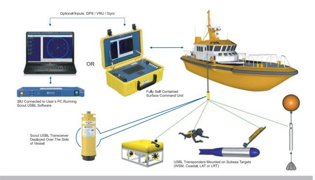
The compact design of the transceiver makes it easy to install on a simple over-the-side mount or through a gate valve. Sonardyne can supply an easy-to-assemble pole, complete with fittings and advice on installation, if required. This ensures the performance of Scout can be optimised for the vessel it is operating from.
