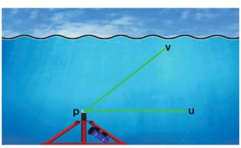
The Aquadopp® can be configured to collect directional wave data at the same time as it measures the mean current. Nortek provides postprocessing software, QuickWave, that uses the PUV method to calculate the full directional wave spectra from the raw data.
