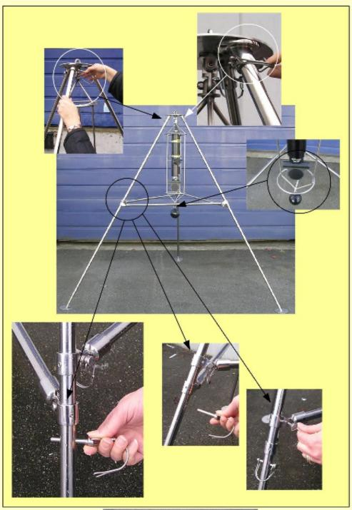
The led weight is supplied to minimize the sonar head from swaying in a current; it does not have to be used if the tripod and head is stable when deployed.
