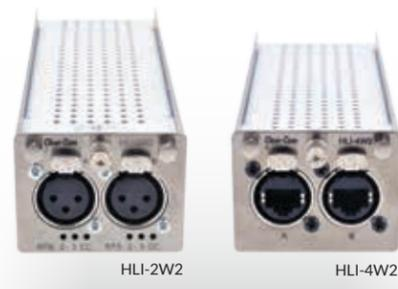
The HLI-4W2 interface module enables 4-wire audio paths, such as matrix ports, cameras and telephone circuits to interface with HelixNet intercom channels. It connects two 4-wire analog audio circuits to HelixNet intercom channels. Two RJ-45 connectors on the module connect the external 4-wire circuits and can be assigned via the main station menu.
