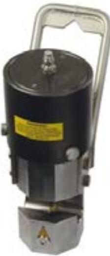
The Webtool 38mm cutter is a hydraulically operated, double acting wire cutter. The RCO40LP can cut wire rope with a minimum 25mm diameter, maximum tensile strength of 1960N/mm up to a maximum 38.1mm diameter with a maximum tensile strength of 1960N/mm.
