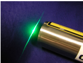
Photo above and right shows laser light in sharp line. Output line fan angle is 80°.
